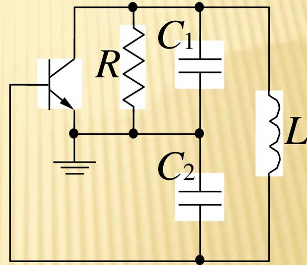
$$\omega_o = \frac{1}{\sqrt{LC_T}} \quad C_T = \frac{C_1 C_2}{C_1 + C_2}$$
